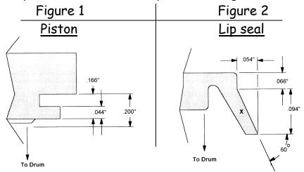
In Reference to Figure 2 (above): With a free lip angle of  $60^{\circ}$  and a lip that is .160" high, the lip has a length of X= .108". With the addition of the .066" of the base above the lip, the maximum height of the seal can only reach .174". This should provide enough clearance for the piston. As you can see in Fig. 1, the height of the groove for the seal to the bottom of the piston is .200". This leaves .026" clearance at the point where the lip is bent to an
